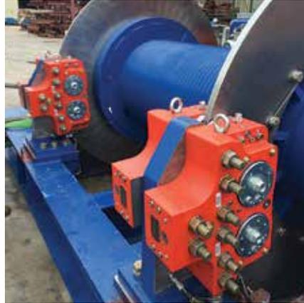
*Two compact, double-piston caliper disc brakes are shown installed on a drawworks drum.*
